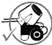
Fig.41: Correct placement of handles for WORKING position.
